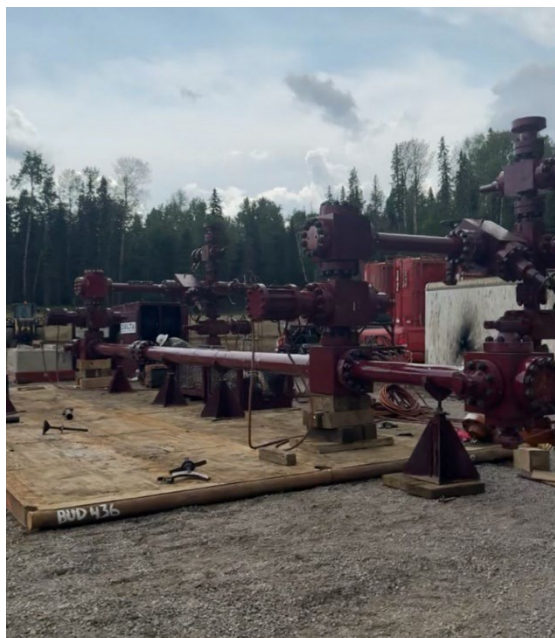
Figure 2 - Surface pressure control system – dual well configuration
